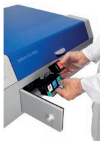
Fig 2. Filters are easily exchanged by the user.
