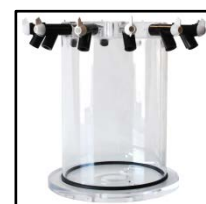
Vertical Drum Manifold
